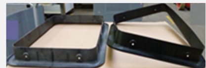
Molded part warpage is lower in XIRAN ® SG grades than in PP-GF. IAC Group warpage comparison on a M.A.N. truck sunroof component.
